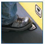
Mounted in the floor plate, the high speed or "rabbit" speed switch gives the T5-72\*\* Tow Tractor series' excellent travel speeds. So whether you're towing one or more carts your operators spend less time traveling, for enhanced productivity and a better bottom line.
