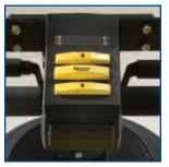
Equipped with a 2-stage electro-mechanical brake, applying the brakes is as easy as squeezing either of the two hand brake levers on the control handle. First-stage applies the Auto Deceleration System. The second stage fully applies the brake. Large push buttons can be operated easily from either side of the steer handle.
