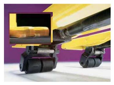
The W60Z forks feature box-rail construction for increased strength and rigidity, throughout its full 6-inches of lift height. Adjustable two-piece heavy-duty pull rod assembly with replaceable threaded ends allow compensation as load wheels wear. Knock-out axles facilitate easy wheel replacement.
