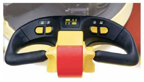
Optional display unit gives you battery state of charge, lift interrupt indication and status codes on an eight character LED screen.
