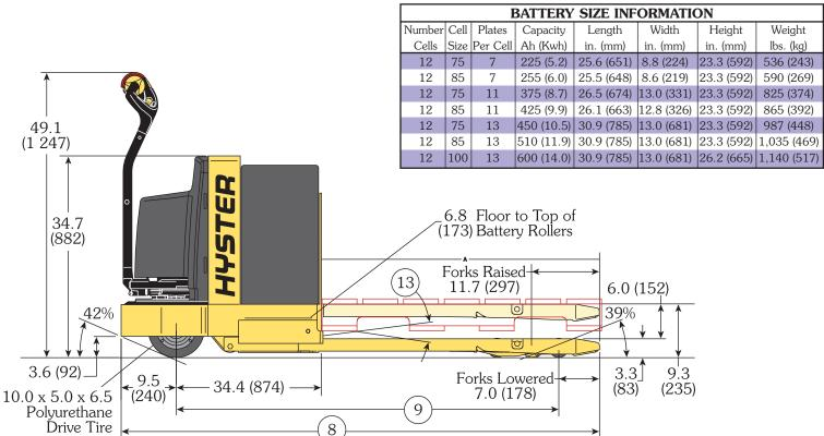
Circled dimensions correspond to the line numbers on the tabulated charts. Dimensions are in inches (millimeters).
