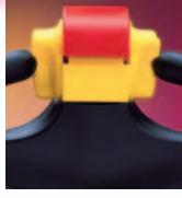
button (brake override), located just below the red direction reversing switch that wraps the end of the handle. It allows you to move the truck with the handle in its fullupright position, to get you into and out of tight spots. The W80Z Walkie Pallet Truck is shown equipped with the optional display that gives you battery state of charge, truck hours, lift interrupt warning and status codes on an eight character LCD screen.
