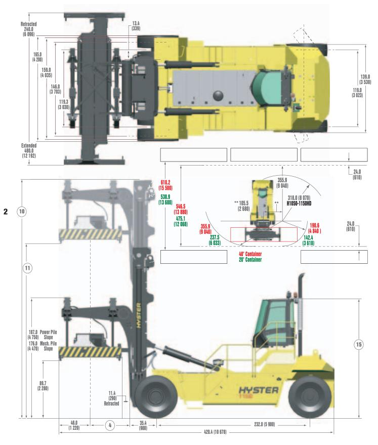
Circled dimensions correspond to the line numbers on the tabulated chart inside the Technical Guide. Dimensions are in inches (millimeters).
